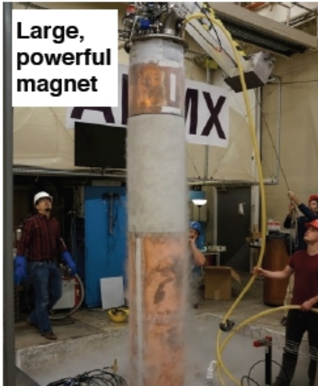
The magnet and microwave cavity convert Milky Way axions into a very weak radio signal
